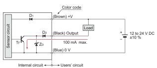
Symbols ... D1: Reverse supply polarity protection diode D2: Reverse output polarity protection diode ZD: Surge absorption zener diode Tr : NPN output transistor
