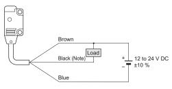
Note: The emitter of the thru-beam type sensor does not incorporate the black wire.
